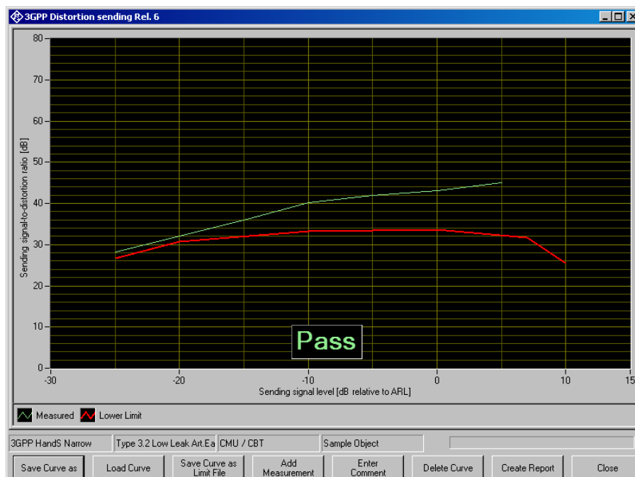
Figure 6-16: Sending distortion measurement
