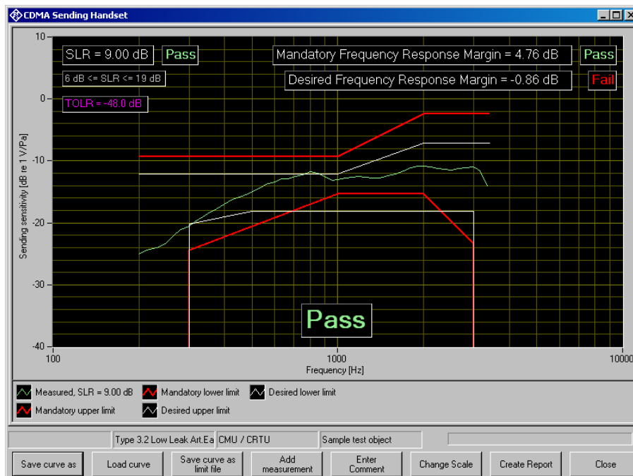
Figure 6-6: Sending frequency response with SLR value displayed
