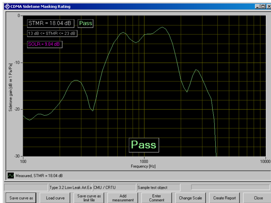
Figure 6-10: Typical Measurement of sidetone masking rating
