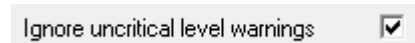
Figure 4-41: Checkbox for suppressing the message caused by excessive single level deviation and other uncritical warnings
