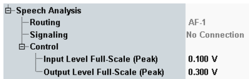
Figure 4-10: Setting of the full-scale peak input and output values in the CMW user interface
