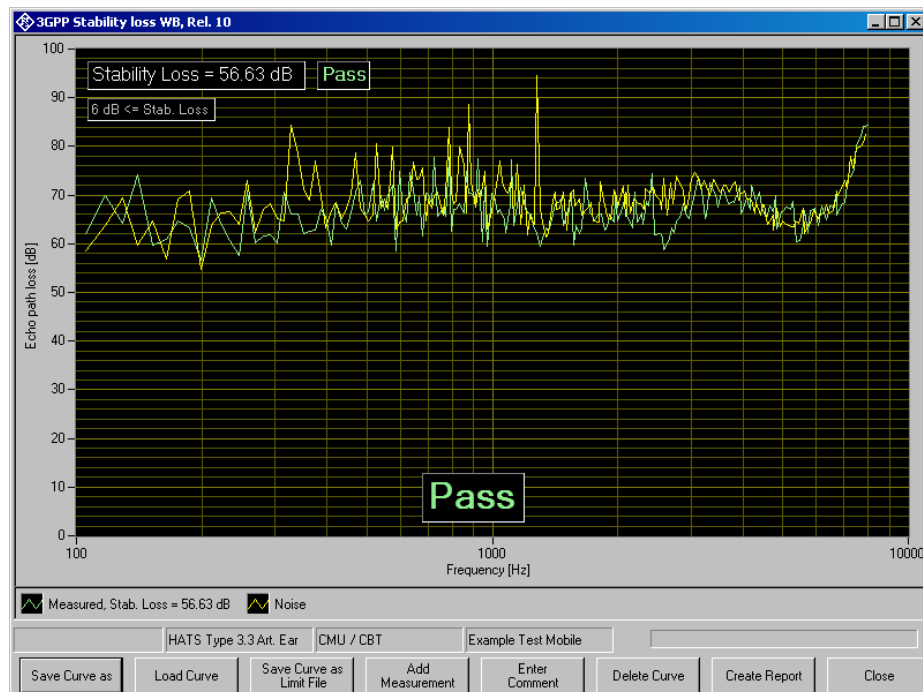
Figure 6-13: Window of stability loss test
